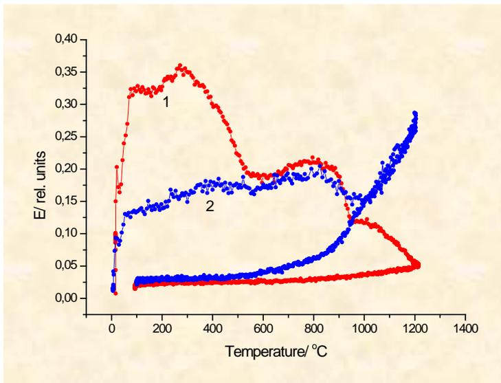
Fig. 3. ETA curves of initial and leaching ceramics: 1 – initial Ca<sub>0,98214</sub> (Nd<sub>0,00790</sub> Ce<sub>0,00996</sub>)Al<sub>0,01786</sub> Ti<sub>0,98214</sub>O<sub>3</sub> – as prepared sample; 2 – sample after hydrothermal treatment at 90°C.
