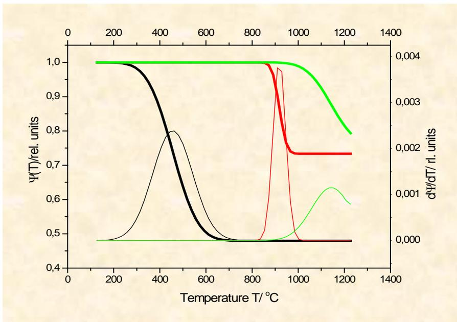
Fig. 4. The structural functions,  $\Psi(T)$  and  $d\Psi/dT$ , designed from ETA
