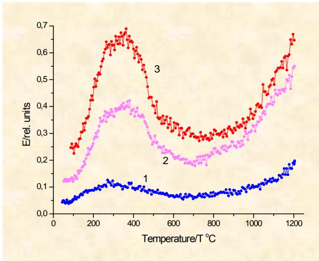
Fig. 2. ETA Perovskite, CaTiO<sub>3</sub>, bombarded 4 MeV krypton ions, linear heating, argon: 1 – initial CaTiO<sub>3</sub>; 2 – CaTiO<sub>3</sub> irradiated by Kr<sup>+</sup> (10<sup>14</sup> ion/cm<sup>-2</sup>); 3 - CaTiO<sub>3</sub> irradiated by Kr<sup>+</sup> (10<sup>15</sup> ion/cm<sup>-2</sup>).
