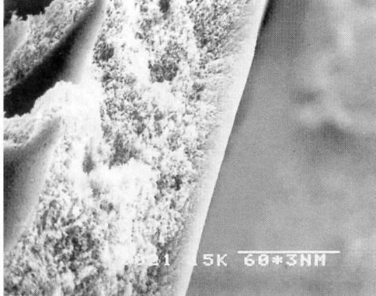
Fig. 1. Gross-section of the PVTMS asymmetric membrane (view of the sublayer)
