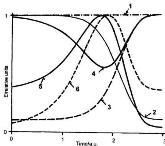
**Fig. 7** Results of the modelling ETA curves characterizing morphology changes on solid state processes at constant temperature. The ‘three components model’ was used in the modelling, the values of emanation rate of individual phases 1, 2 and 3 are given in Table 1 as  $E_1$ ,  $E_2$  and  $E_3$
