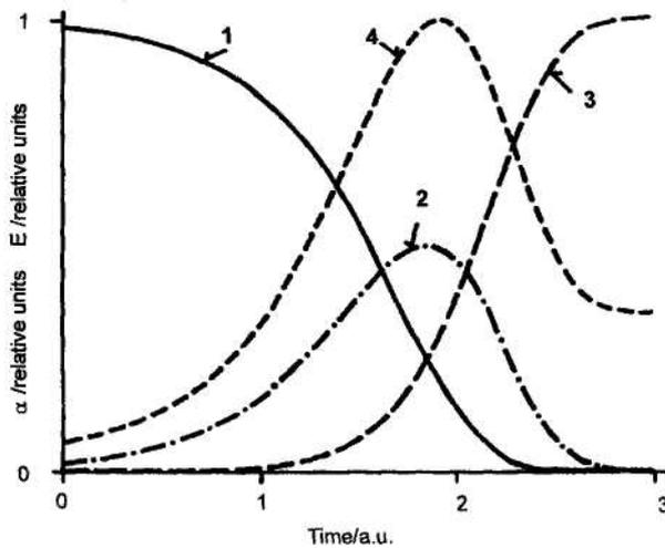
**Fig. 6** Time dependences of the concentrations of individual phases 1, 2 and 3 (curves 1, 2 and 3, resp.) involved in the ‘three components model’ of hydration. The theoretical ETA curve calculated by means of the model is given as curve 3
