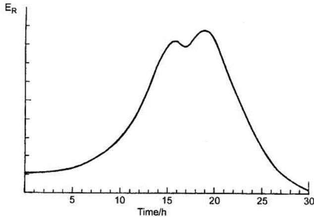
**Fig. 5** Simulated curve of the emanation rate measured during hydration of  $3\text{CaO}\cdot\text{SiO}_2$  at 293 K ( $w/\text{solid}=0.4$ ) supposing a two-sized calcium silicate sample (grain sizes 0.7 and 3.5  $\mu\text{m}$ )
